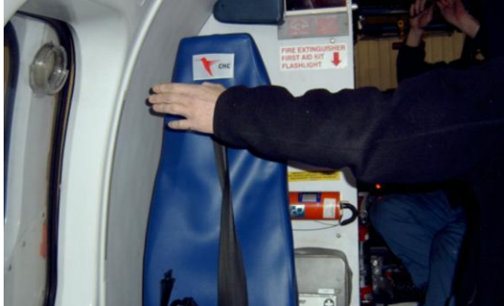
Figure 5. AS332L forward passenger seat of auxiliary fuel tank. ( Note: the passenger must egress across the aisle ).
