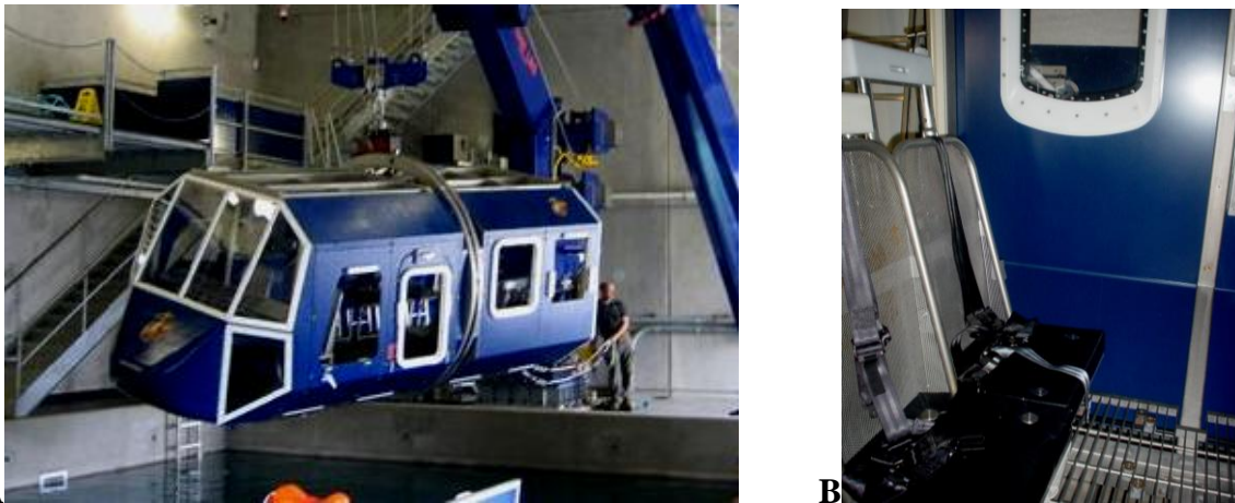
Figure 8. METST TM model 40 showing 4 different exit types (Panel A). Interior of METST TM showing high-back crashworthy seats fully compressed and 4-point harnesses (Panel B).
